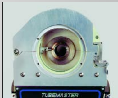
Collets removed to show Fillet Weld
